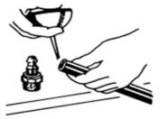
III Lubricate the inside of the hose with a little light engine oil. Place the hose on the spigot and then firmly push the hose home until it butts up against the end stop of the fitting. This may require some force, particularly with the larger sizes of hose,
